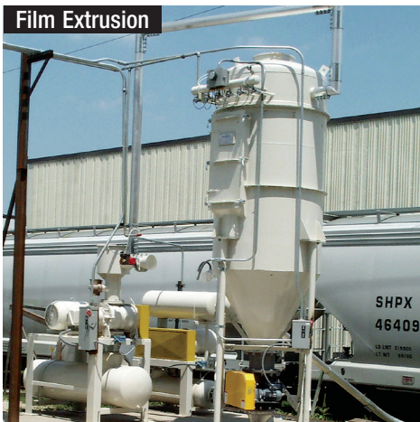
Rail car unload system
