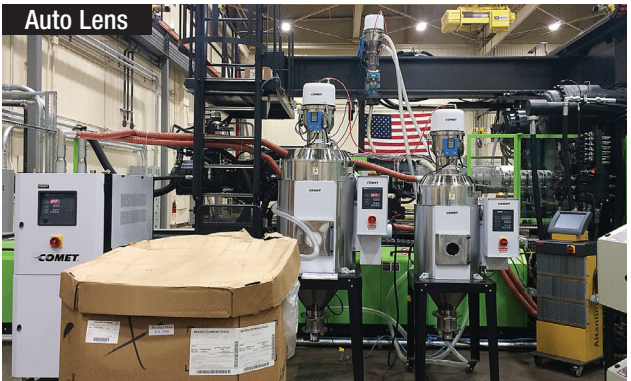
CD-300 honeycomb matrix dryer, three CHD dryer hoppers, and CAL hopper loaders on a 3-color Engel machine
