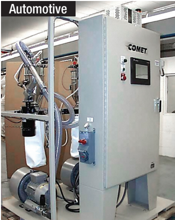
Allen-Bradley conveying control has automatic backup pump, filter, and relief valve for tube extrusion
