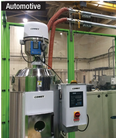
CHD dryer hopper and CAL hopper loaders
