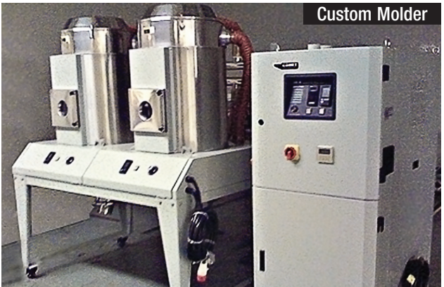
CD honeycomb matrix dryer with two CHD drying hoppers and separate drying controls
