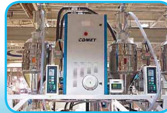
Honeycomb Dryer with Two (2) Drying Hoppers
