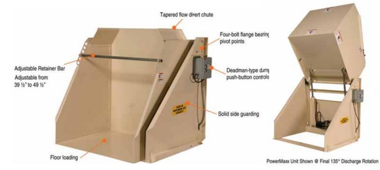
Comet's PowerMaxx Container Discharger is easy to install and use. It is designed to reduce labor and operation costs by safely transferring plastic material from a wide variety of container shapes and sizes into storage bins or processing equipment. By manually pressing and holding the raise/lower selector switch, the PowerMaxx can take containers at floor level and invert them 45° with a total rotation of 135°.
