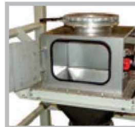
Opened access door & safety switch disengaged
