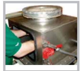
Operator is safely accessing the bag's discharge spout to untie and/or re-tie the spout
