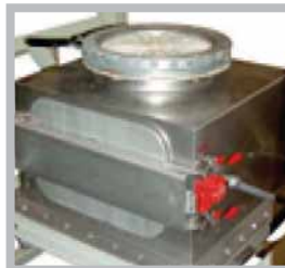
Closed access door with safety switch engaged
