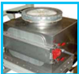
Closed access door with safety switch engaged
