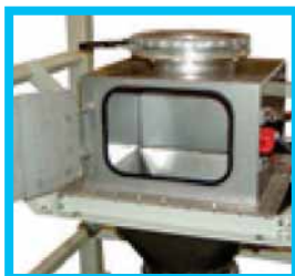
Opened access door & safety switch disengaged
