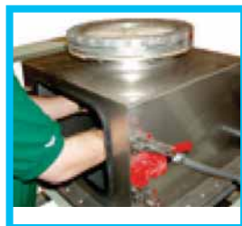
Operator is safely accessing the bag's discharge spout to untie and/or re-tie the spout
