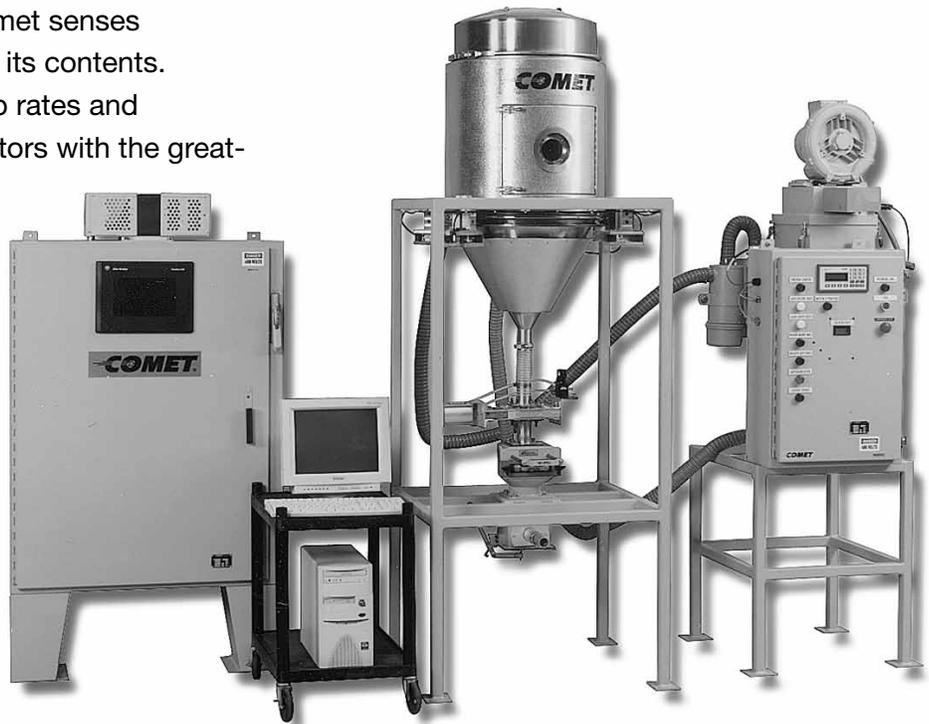
The interface provides virtually unlimited storage of process data on a standard PC and enables users to customize reports, print charts and graphs of material usage, dryer temperature, dewpoint, etc.
