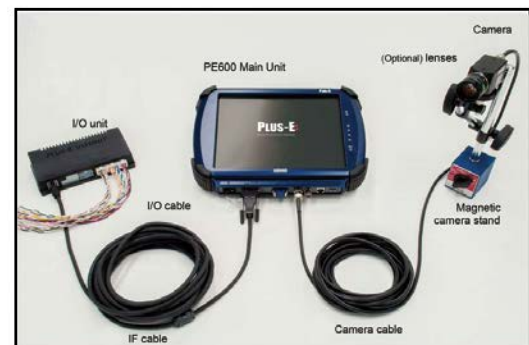
Connecting Example for Standard Set
