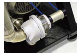
Vacuum Breaking Valve
