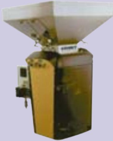
The Comet GraviMix™ blender is designed to blend free-flowing pellets in processes which require accurate dosing and repeatability with efficient mixing. Unaffected by vibrations, this unit mounts easily onto the throat of the processing machine, to be installed either on a mezzanine, or on a vacuum take-off stand to feed one or more machines.
