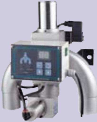
Comet's Two-Component CPV proportioning valve enables two materials to be conveyed in a preselected percentage through an individual hopper loader or a central vacuum receiver. Through in-line mixing, the CPV eliminates virgin and regrind layering, common in ratio loaders. Material proportion can be digitally set on the electronic control box mounted on the unit. During a single conveying cycle, it is possible to switch materials (virgin and regrind) as often as desired.
