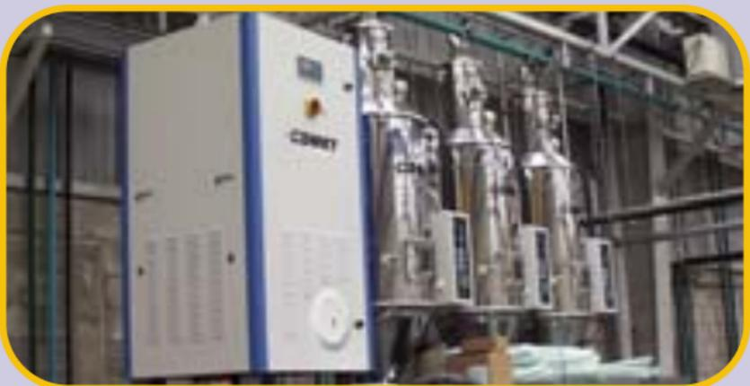
*Centralized Honeycomb Drying System*
