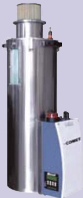
Comet's ERD Xpert uses dehumidified compressed air from the plant's air system for the drying process. This unique system requires no maintenance and is the most efficient way to dry small batches of material.
