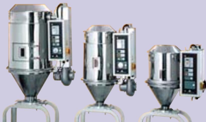
Comet's CDH-Series hot air dryer, dries plastic granules directly at the machine eliminating contamination or re-absorption of moisture when conveying from a central drying position to a machine hopper. This dryer is ideally suited for continuous drying from 5 - 600 lbs. per hour of plastic granules.
