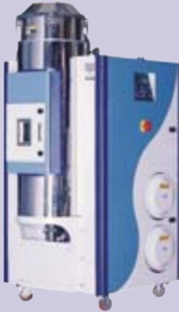
The compact dryer, mounted on a mobile frame, consists of three main parts: the Honeycomb Dehumidified Dryer, the Drying Hopper and the Loading System. The loaders feed to and from the drying hopper to the machine or, as an option, from the surge bin to the drying hopper. The FCD can supply one material to six machines and, depending on production requirements, special loaders can be designed to handle powder and dust separation. The vacuum pump and fines filter are mounted inside the unit.
