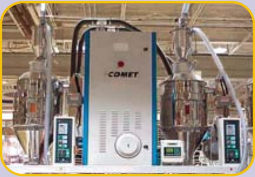
*Honeycomb Dryer with 2 Drying Hoppers*
